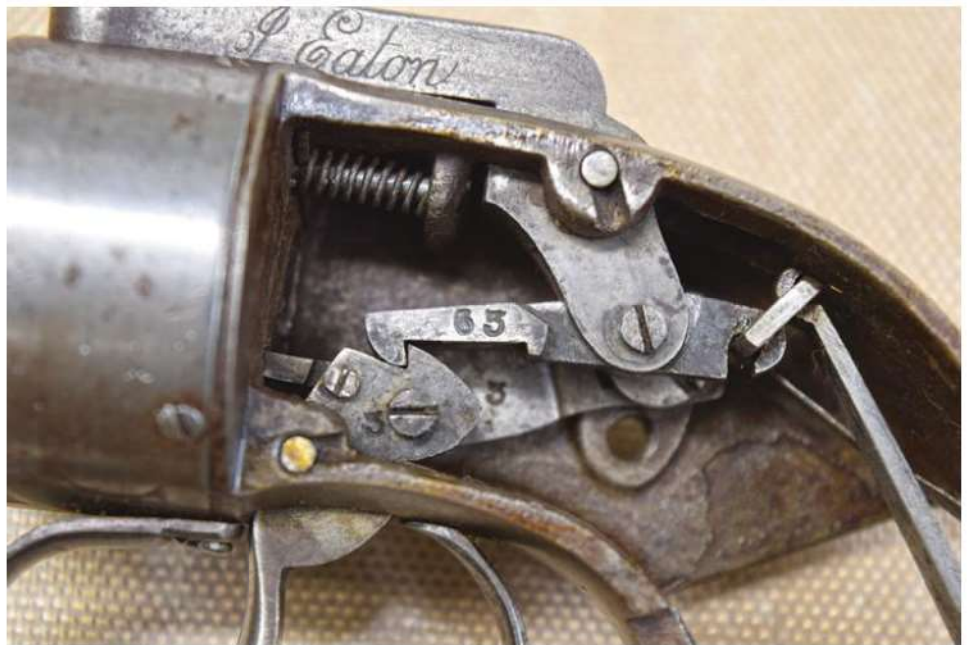
A double action Pepperbox derringer made by Allen and Thurber during the middle of the 19th century. It belongs to Death Valley National Park. The images show it before treatment and then disassembled during treatment, allowing all of the internal information and condition to be documented and treated / NPS photos
