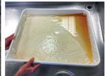
Water after bathing a very acidic paper object. The discoloration removed from the paper comes from acidic components in the paper pulp which darken over time and threaten the stability of the paper. The treatment can make the paper stronger and slow further deterioration.
